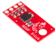
Figura 29 – IMU SparkFun 9DoF Sensor Stick da empresa SparkFun
